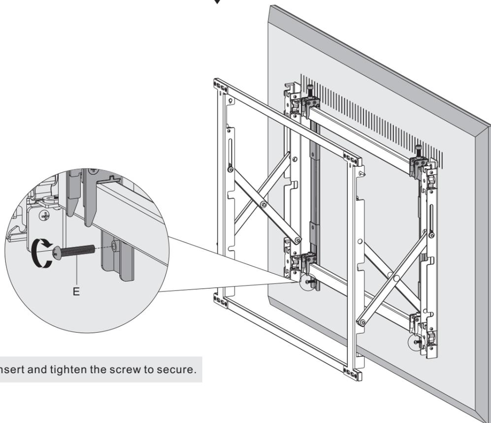
Insert and tighten the screw to secure.
