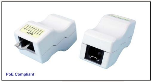
LOKJAC Category 6 Locking Inline Coupler, shielded (SACSLJ) and unshielded (SACLJ) These LOKJAC locking couplers enable cables to be easily extended and sockets to be temporarily relocated. The locking/blocking facility prevents unauthorised use of the connection and avoids unintended disconnection where vibration or interference is a concern.
