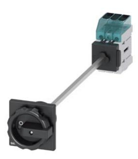
Switch disconnector 3LD3, main switch 3-polig, lu 25A operational switch at AC-23 A at 400 V 9,0 kW floor mounting Base mounting with door coupling center-hole 22,5 mm rotary operationg mechanism black  $66 \times 66$  mm
