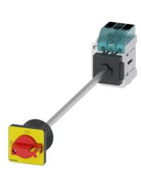
Switch disconnector 3LD3, main switch 3-polig, lu 32A operational switch at AC-23 A at 400 V 11,5 kW floor mounting Base mounting with door coupling center-hole 22,5 mm knob-operated mechanism red/yellow 48 x 48 mm with auxiliary 1NO+1NC
