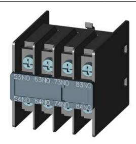
AUX.SWITCH BLOCK,FRONT,4NO, CURR.PATH: 1NO, 1NO, 1NO, 1NO, FOR CONTACTOR RELAYS, SZ S00, RING CABLE LUG CONNECTION 53 / 54,63 / 64,73 / 74,83 / 84
