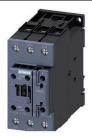
CONTACTOR,AC3:30KW/400V, 1NO+1NC, 220V AC 60HZ, 3-POLE, SIZE S2, SCREW TERMINAL
