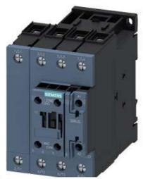
4NO CONTACTOR,AC1:60A 175-280V AC/DC,VARISTOR, 4-POLE, 4NO, SIZE S2, SCREW TERMINAL 1NO+1NC INTEGRATED
