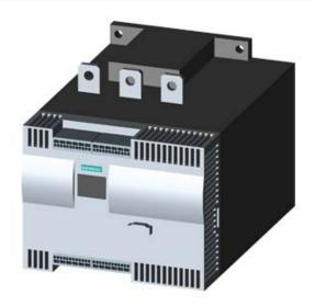
SIRIUS SOFT STARTER, VALUES WITH 400 V, 40 DEG., STANDARD: 203A, 110KW, INSIDE-DELTA CIRCUIT 3: 352A, 200KW, 200-460 V AC, 230 V AC, CAGE CLAMP TERMINALS
