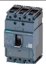
CIRCUIT BREAKER 3VA1 IEC FRAME 160 BREAKING CAPACITY CLASS N ICU=25KA @ 415 V 3-POLE, LINE PROTECTION TM220, ATFM, IN=16A OVERLOAD PROTECTION IR=11,2A ...16A SHORT CIRCUIT PROTECTION II=10 X IN CABLE CONNECTION
