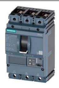
CIRCUIT BREAKER 3VA2 IEC FRAME 160 BREAKING CAPACITY CLASS C ICU=110KA @ 415 V 3POLE, LINE PROTECTION ETU860, LSIG, IN=160A OVERLOAD PROTECTION IR=64A ...160A SHORT CIRCUIT PROTECTION ISD=0,6..10X IN, II=1,5..10X IN NEUTRAL PROTECTION OPTIONAL WITH EXT. CT,UPTO 160% GROUNDFAULT, SWITCHABLE IG=0,2... 1 X IN, TG=0,050,8MS BUSBAR CONNECTION
