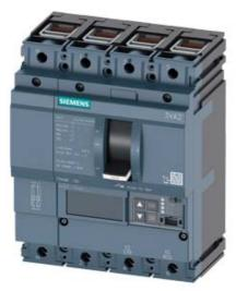
CIRCUIT BREAKER 3VA2 IEC FRAME 160 BREAKING CAPACITY CLASS C ICU=110KA @ 415 V 4POLE, LINE PROTECTION ETU850, LSI, IN=40A OVERLOAD PROTECTION IR=16A ...40A SHORT CIRCUIT PROTECTION ISD=0,6..10X IN, II=1,5..12X IN NEUTRAL PROTECTION ADJUSTABLE (OFF, UPTO 160%) CABLE CONNECTION
