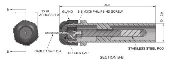
A single pole electrode used for level control in wells or storage tanks. It comprises of stainless steel Sensor with plastic holder and cable gland. A sealed ring and cable gland prevents liquid from entering the cable terminal connector and causing its oxidation. Maximum operating temperature: -10°C to + 65°CCable connection: Screw The external cable diameter must be 1.5 mm to warrant perfect sealing.
