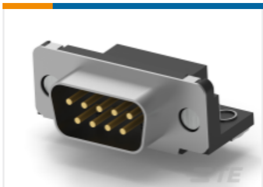
TE Part #1-338168-2 D-Sub Plug Assembly: Standard, Right Angle, Shell Size 1, 2.74mm
