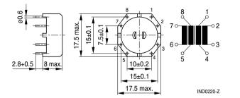
Tolerances to ISO 2768-M unless otherwise noted. Dimensions in mm.
