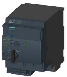
SIRIUS, COMPACT STARTER, REVERSING STARTER . 690 V, 24 V DC, 1 ... 4 A, IP20, CONN. MAIN CIRCUIT: PLUG-IN, W/O TERMINALS, CONN. CONTROL CIRCUIT: SPRING-LOADED TERMINAL
