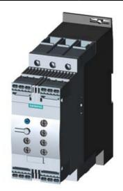
SIRIUS SOFT STARTER, S2, 45A, 22KW/400V, 40 DEGR., AC 200-480V, AC/DC 24V, SPRING-LOADED TERMINALS, THERMISTOR MOTOR PROTECTION
