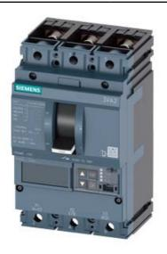
CIRCUIT BREAKER 3VA2 IEC FRAME 100 BREAKING CAPACITY CLASS H ICU=85KA @ 415 V 3POLE, LINE PROTECTION ETU560, LSIG, IN=40A OVERLOAD PROTECTION IR=16A ...40A SHORT CIRCUIT PROTECTION ISD=0,6..10X IN, II=1,5..12X IN NEUTRAL PROTECTION OPTIONAL WITH EXT. CT,UPTO 160% GROUNDFAULT, SWITCHABLE IG=0,2... 1 X IN, TG=0,050,8MS BUSBAR CONNECTION
