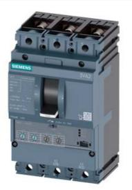
CIRCUIT BREAKER 3VA2 IEC FRAME 160 BREAKING CAPACITY CLASS C ICU=110KA @ 415 V 3POLE, LINE PROTECTION ETU350, LSI, IN=63A OVERLOAD PROTECTION IR=25A ...63A SHORT CIRCUIT PROTECTION ISD=1,5... 10 X IR, II=12 X IN BUSBAR CONNECTION
