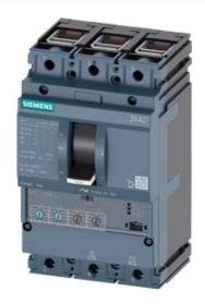
CIRCUIT BREAKER 3VA2 IEC FRAME 160 BREAKING CAPACITY CLASS C ICU=110KA @ 415 V 3POLE, LINE PROTECTION ETU350, LSI, IN=63A OVERLOAD PROTECTION IR=25A ...63A SHORT CIRCUIT PROTECTION ISD=1,5... 10 X IR, II=12 X IN CABLE CONNECTION
