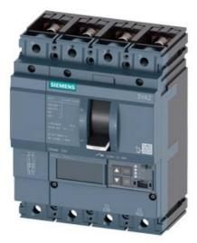
CIRCUIT BREAKER 3VA2 IEC FRAME 250 BREAKING CAPACITY CLASS C ICU=110KA @ 415 V 4POLE, LINE PROTECTION ETU550, LSI, IN=160A OVERLOAD PROTECTION IR=64A ...160A SHORT CIRCUIT PROTECTION ISD=0,6..10X IN, II=1,5..12X IN NEUTRAL PROTECTION ADJUSTABLE (OFF, UPTO 160%) BUSBAR CONNECTION
