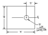
Thermasil III electrically insulating pad with adhesive backing for a TO-220 device. Composed of a silicone elastomer binder with a thermally conductive filler and reinforced with finely woven glass cloth to resist tearing.
