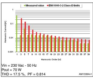
Figure 5. EVL4984-350W: compliance with JEITA-MITI standard at 70 W load
