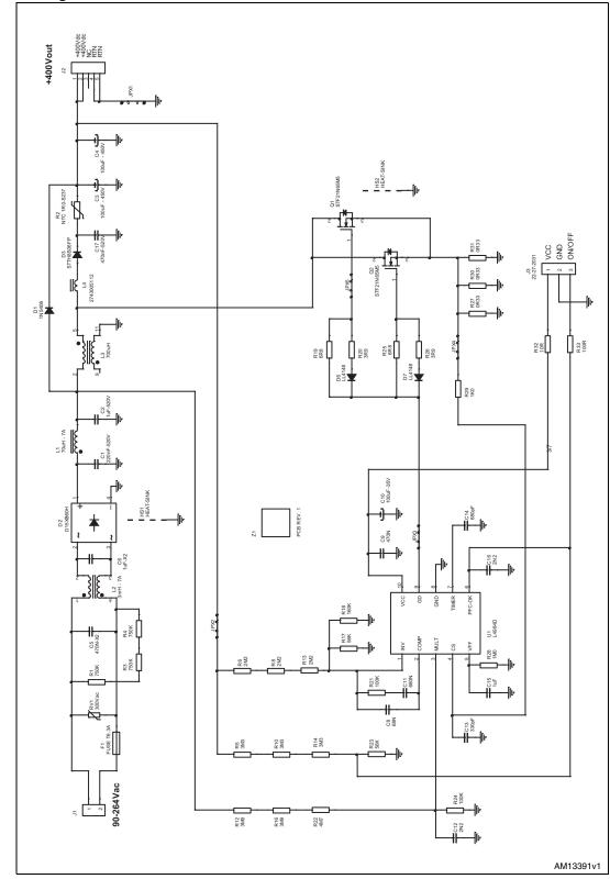
Figure 1. EVL4984-350W CCM PFC demonstration board electrical schematic
