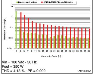
Figure 4. EVL4984-350W: compliance with EN61000-3-2 standard at 70 W load
