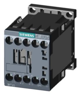
CONTACTOR, AC-3, 5.5KW/400V, 1NC, DC 24V, W. INTEGRATED DIODE 3-POLE, SZ S00 SCREW TERMINAL
