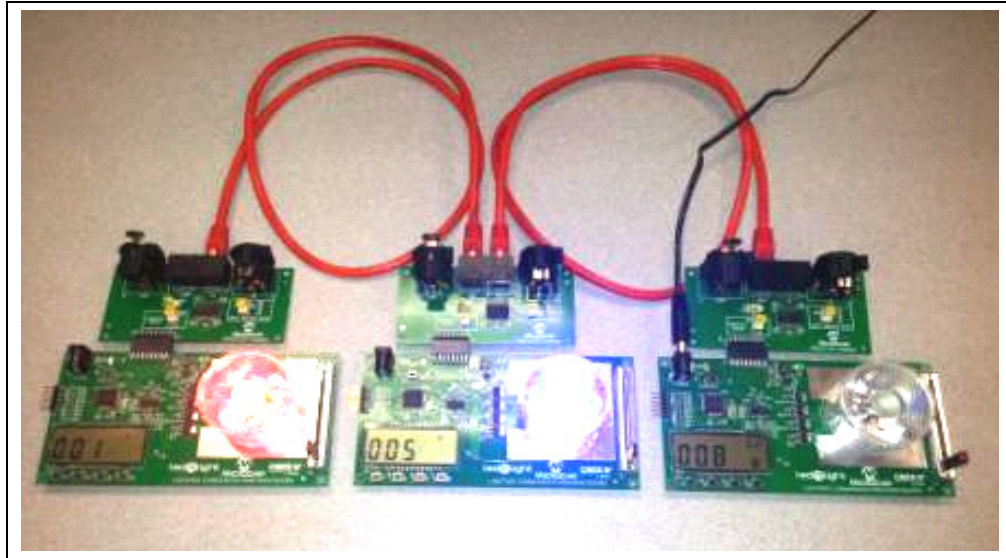
FIGURE 5-4: DMX512A DEMONSTRATION CONFIGURATION
