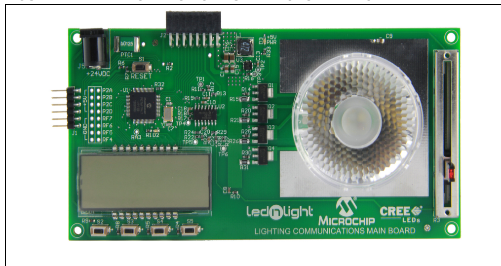
FIGURE 2-1: LIGHTING COMMUNICATIONS MAIN BOARD
