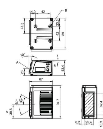
A Optical axis B M4 thread (5 deep) Part no.: 50141828 – BCL 338i SF 102 D F007 – Stationary bar code reader
