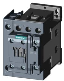
2S+2OE SCHUETZ, AC3: 11KW AC 24V 50/60HZ 4-POLIG, 2S+2OE, BGR: S0, SCHRAUBANSCHLUSS 1S+1OE INTEGR.
