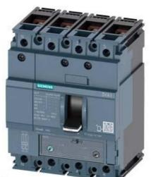
CIRCUIT BREAKER 3VA1 IEC FRAME 160 BREAKING CAPACITY CLASS M ICU=55KA @ 415 V 4-POLE, LINE PROTECTION TM240, ATAM, IN=125A OVERLOAD PROTECTION IR=87,5A ...125A SHORT CIRCUIT PROTECTION II=5...10 X IN NEUTRAL PROTECTION 100% BUSBAR CONNECTION
