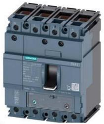
CIRCUIT BREAKER 3VA1 IEC FRAME 160 BREAKING CAPACITY CLASS N ICU=25KA @ 415 V 4-POLE, LINE PROTECTION TM240, ATAM, IN=20A OVERLOAD PROTECTION IR=14A ...20A SHORT CIRCUIT PROTECTION II=5...10 X IN NEUTRAL UNPROTECTED CABLE CONNECTION
