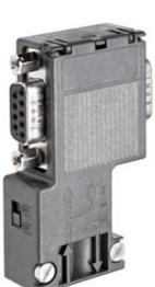
PROFIBUS bus connector, RS485, screw, with PG socket, 90° PROFIBUS bus connector, RS485, srew, with PG socket, 90° SIMATIC DP, BUS CONNECTOR FOR PROFIBUS UP TO 12 MBIT/S 90 DEGREE ANGLE CABLE OUTLET, 15,8 X 64 X 35,6 MM (WXHXD), TERMINAT. RESIST. WITH ISOLAT. FUNCTION, WITH PG SOCKET
