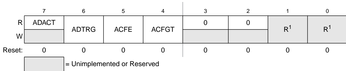
Figure 9-5. Status and Control Register 2 (ADCSC2)
