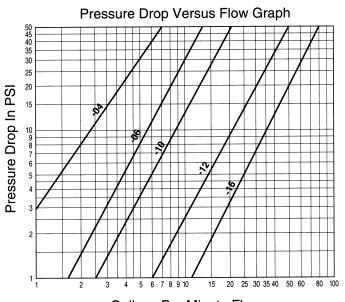
Gallons Per Minute Flow (Test Fluid MIL-H-5606 Hydraulic Oil At 100° F.)
