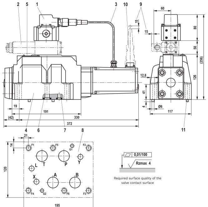
Device dimensions size 25 (dimensions in mm)
