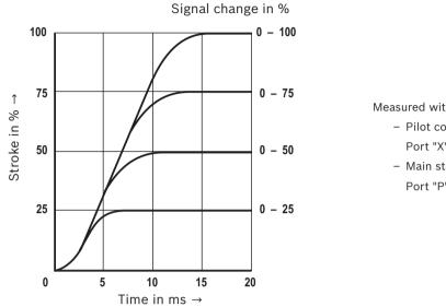
Measured with: - Pilot control valve Port "X" = 140 bar - Main stage Port "P" = 10 bar
