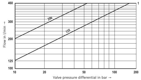
**1** = recommended flow limitation (flow velocity 30 m/s)
