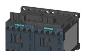
REV. COMB., AC3, 4KW/400V AC48V, 50/60 HZ, 3-POLE, SZ S00 SCREW TERMINAL ELECTR. AND MECH. INTERLOCK
