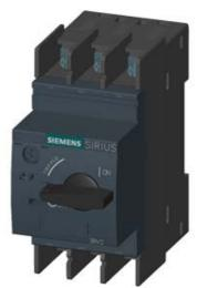
CIRCUIT-BREAKER SZ S00, FOR MOTOR PROTECTION, CLASS 10, A-RELEASE 4.5...6.3A, N-RELEASE 82A RING CABLE LUG CONNECTION, STANDARD SW. CAPACITY
