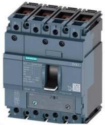
CIRCUIT BREAKER 3VA1 IEC FRAME 160 BREAKING CAPACITY CLASS N ICU=25KA @ 415 V 4-POLE, LINE PROTECTION TM240, ATAM, IN=16A OVERLOAD PROTECTION IR=11,2A ...16A SHORT CIRCUIT PROTECTION II=5 X IN NEUTRAL PROTECTION 100% BUSBAR CONNECTION
