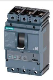
CIRCUIT BREAKER 3VA2 IEC FRAME 160 BREAKING CAPACITY CLASS M ICU=55KA @ 415 V 3POLE, LINE PROTECTION ETU330, LIG, IN=63A OVERLOAD PROTECTION IR=25A ...63A SHORT CIRCUIT PROTECTION II=1,5...12 X IN GROUNDFAULTPROTECTION IG=0,2... 1 X IN, TG=0,1/0,3MS BUSBAR CONNECTION
