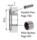
The thrust washer must be secured against rotation, with a parallel pin or with adhesive.
