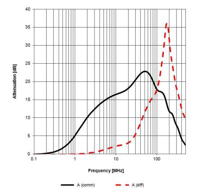
**F** Typical Insertion Loss Characteristics:
