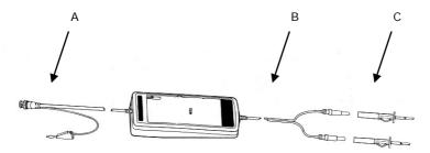
A. Output Lead The BNC output connector and an auxiliary grounding terminal are connected to the oscilloscope.
