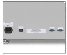
Interface for data transmission from the SAUTER FH measuring device and for controlling the test stand with SAUTER AFH software
