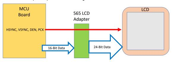
The following figure shows the color mapping from a 16-bit source output from the microcontroller, where 24-bit is the input to an LCD panel. The lower LSBs of the 24-bit connections are tied to the MSB from the 16-bit output. This allows the maximum color output on the LCD panel when the 16-bit value is written to the maximum of its output space.
