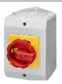
MAIN/EMERG. STOP SWITCH 3-POLE IU=63 P/AC-23A AT 400V=22KW SWITCH IN ISO ENCLOSURE ROTARY ACTUATOR RED/YELLOW (EMERG. STOP) PE-TERMINAL MOUNTED ON SWITCH
