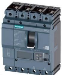
CIRCUIT BREAKER 3VA2 IEC FRAME 100 BREAKING CAPACITY CLASS L ICU=150KA @ 415 V 4POLE, LINE PROTECTION ETU850, LSI, IN=63A OVERLOAD PROTECTION IR=25A ...63A SHORT CIRCUIT PROTECTION ISD=0,6..10X IN, II=1,5..12X IN NEUTRAL PROTECTION ADJUSTABLE (OFF, UPTO 160%) BUSBAR CONNECTION
