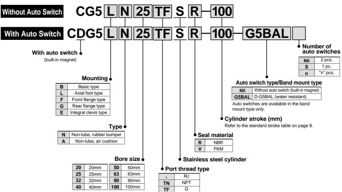
Bore size-Ø 20-25mm available in port thread M only for air
