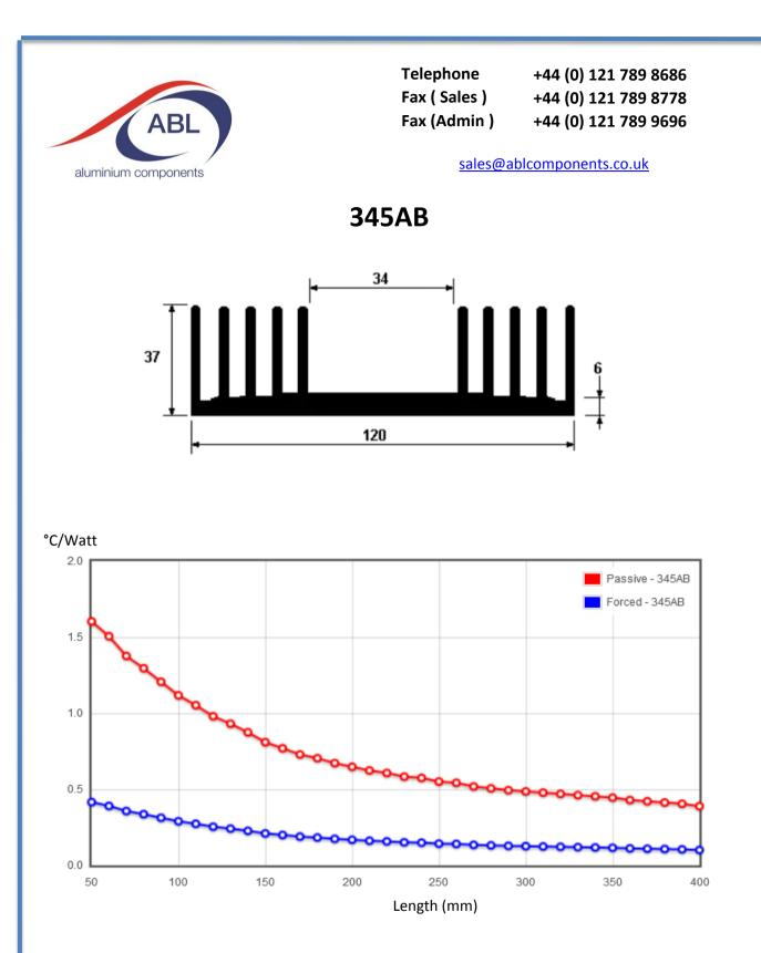
Thermal Resistance is calculated based on a distributed heat load and vertically mounted fins anodised heatsink with a 60°C temperature.
