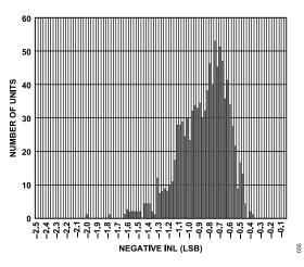
Figure 25. Typical Negative INL Distribution (999 Units)
