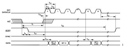
Figure 8. Conversion and Read Timing for Reading Previous Conversion Results During A Conversion Using External Discontinuous Data Clock (EXT/ INT Set to Logic High, CS Set to Logic Low)
