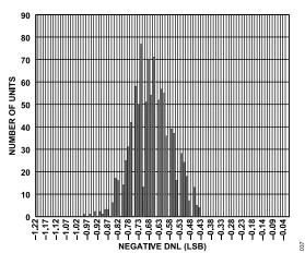
Figure 27. Typical Negative DNL Distribution (999 Units)
