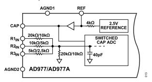
Figure 13. AD977/AD977A Simplified Analog Input
