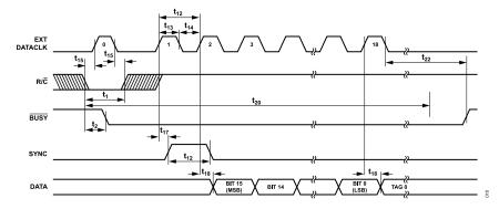
Figure 10. Conversion and Read Timing for Reading Previous Conversion Results During a Conversion Using External Discontinuous Data Clock (EXT/ INT Set to Logic High, CS Set to Logic Low)
