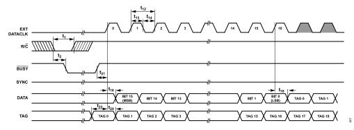
Figure 7. Conversion and Read Timing Using an External Discontinuous Data Clock (EXT/INT Set to Logic High, CS Set to Logic Low)
