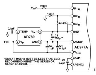
Figure 20. AD780 External Reference to AD977A Configured for ±10 V Input Range
