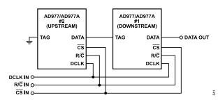
Figure 31. Two AD977/AD977A's Utilizing Tag
