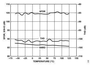
Figure 29. AC Parameters vs. Temperature
