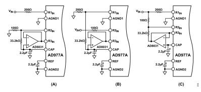
Figure 14. AD977A Bipolar Input Configuration Using the Internal Reference; (a) V<sub>IN</sub> = ±10 V, (b) V<sub>IN</sub> = ±5 V, (c) V<sub>IN</sub> = ±3.33 V
