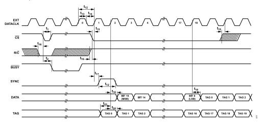
Figure 11. Conversion and Read Timing Using an External Continuous Data Clock (EXT/ INT Set to Logic High)
