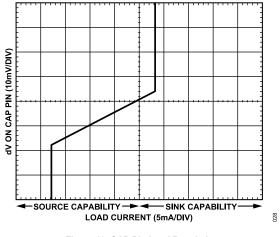
Figure 18. CAP Pin Load Regulation
