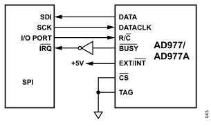
Figure 33. AD977/AD977A to SPI Interface
