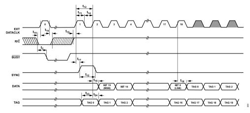
Figure 9. Conversion and Read Timing Using An External Discontinuous Data Clock (EXT/INT Set to Logic High, CS Set to Logic Low)
