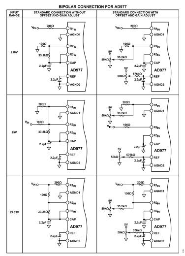
Figure 15. AD977 Bipolar Analog Input Configuration
