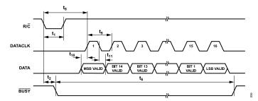
Figure 6. Serial Data Timing for Reading Previous Conversion Results with Internal Clock (CS, EXT/INT and TAG Set to Logic Low)
