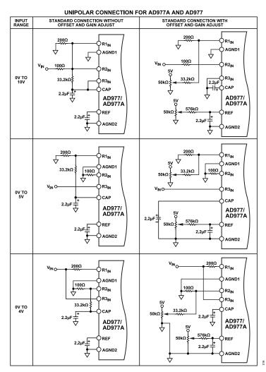
Figure 16. AD977/AD977A Unipolar Analog Input Configuration
