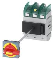
SENTRON, Molded case switch 3LD5 UL, Emergency switching-off, 3-pole, certified according to UL489 UL60947-4-1 and IEC60947-3, UL: 150A, SCCR 50kA at 480VAC, Operating power at 480VAC 3-phase: 100hp, IEC: 160A, Operating power at AC-23A at 400V: 75kW, floor mounting with door coupling rotary operating mechanism, defeatable, emergency switching-off, 4-hole mounting of the handle, without tolerance compensation, incl. terminal covers for the infeed side
