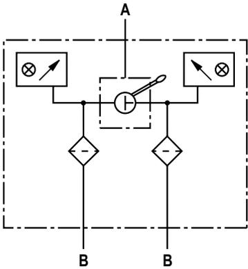
**Tank mounted return line filter without bypass and with mechanical indicator**
