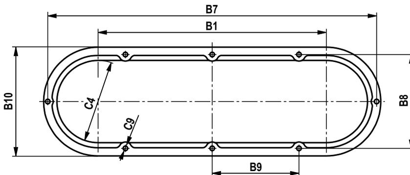
Hole pattern tank cover (1/2 shown) without installation plate
