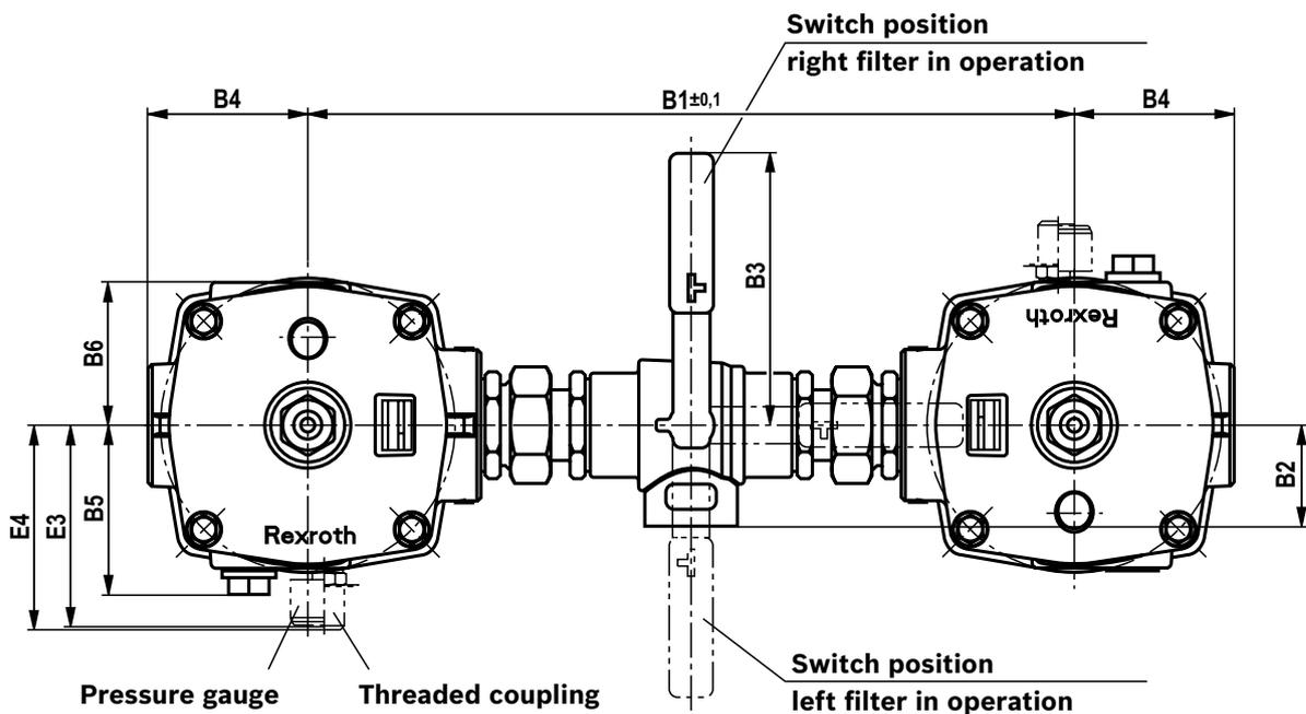
1) Observe the servicing height plus the length of the outlet pipe, if applicable
