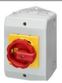
EMERG. STOP SWITCH 3-POLE IU=25, P/AC-23A AT 400V=9.5KW 1NO+1NC, 1 N-TERMINAL INSULATION-ENCLOSED, IP65 ROTARY ACTUATOR RED/YELLOW (EMERG. STOP) METRIC SCREW CONNECTION
