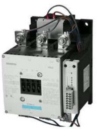
CONTACTOR, 110KW/400V/AC-3 AC(40...60HZ)/DC OPERATION UC 96-127V AUXILIARY CONTACTS 1NO+1NC 3-POLE, SIZE S10 BAR CONNECTIONS ELECTRONIC OPERATING MECHANISM WITH PLC/SIMOCODE INTERFACE AND REMAIN. LIFETIME INDICATOR
